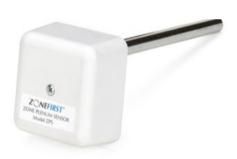
The ZPS inserts into the supply air duct, see location information and drawing below, and requires only two (2) wires to the zoning panel. Lengths longer than 15 feet or that come in close contact with line voltage, shielded cable is recommended.
