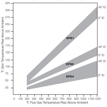
NOTE: The Outer Jacket Temperature Rise chart is intended to be a guide only. It is indicative of the likely outer jacket temperatures for any particular PowerStack application, but cannot be exact as each situation requires a calculation and knowledge of mass flow, velocity of the gases, and the location and situation of the chimney, i.e.: enclosed non-ventilated, enclosed ventilated, not enclosed, external, etc.
