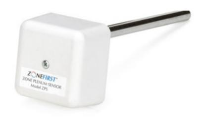
The ZPS inserts into the supply air duct, see location information and drawing below, and requires only two (2) wires to the zoning panel. Lengths longer than 15 feet or that come in close contact with line voltage, shielded cable is recommended.
